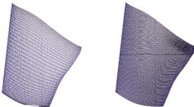
Fig. 5 (a) Source mesh: 43 sections with 89 nodes; (b) mesh used for resection: 172 sections with 89 nodes
