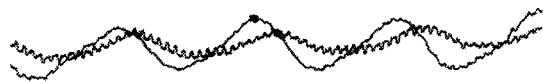
Fig. 11 Kulite data from the rotor platform. The root injection (jagged line) shows noticeable wake reduction from the non-cooled case. Four vane passages are shown.
